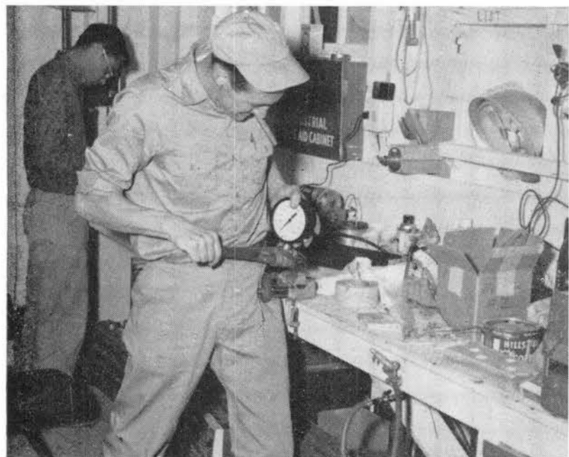
PRESSURE in Gnome cavity after the nuclear detonation will be measured by equipment being assembled in Sandia trailer at Gnome site by J. A. Kastening (7251-2), left, and J. A. Beyeler (7251-3). Gas pressure in cavity after blast is expected to be in the order of several hundred pounds per square inch.
